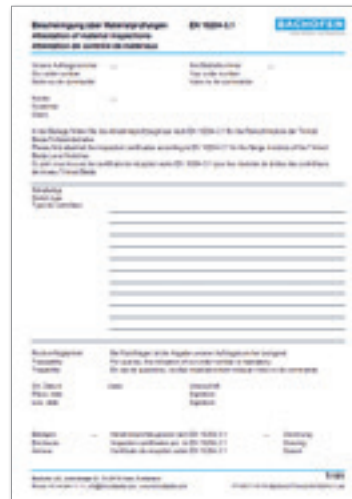
Inspection certificate 3.1 acc. to EN 10204 For flange materials of the level switches, counterflanges and the intermediate part of the test actuators.
